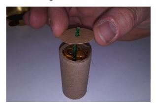
10. After the round is cool, trim the fuse to a length of  $\frac{1}{4}$ " at a 45° angle.
